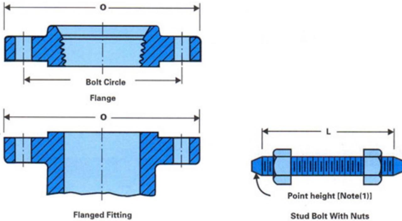
TABLE 17 TEMPLATES FOR DRILLING CLASS 600 FLANGES<sup>2</sup>
