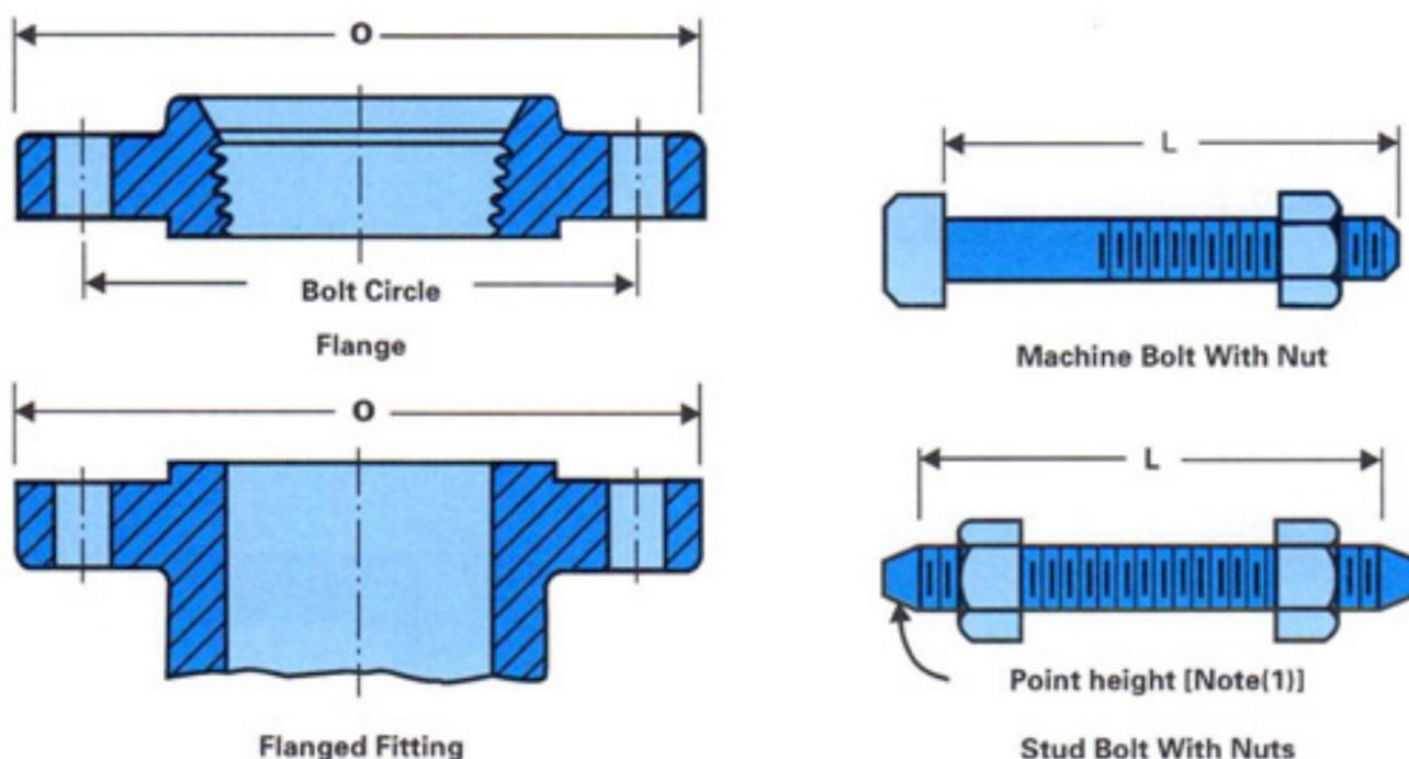
TABLE 8 TEMPLATES FOR DRILLING CLASS 150 FLANGES<sup>2</sup>
