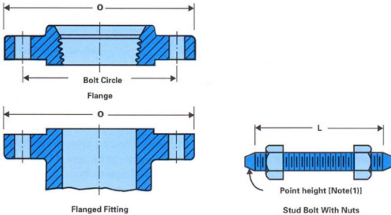
TABLE 26 TEMPLATES FOR DRILLING CLASS 2500 FLANGES<sup>2</sup>
